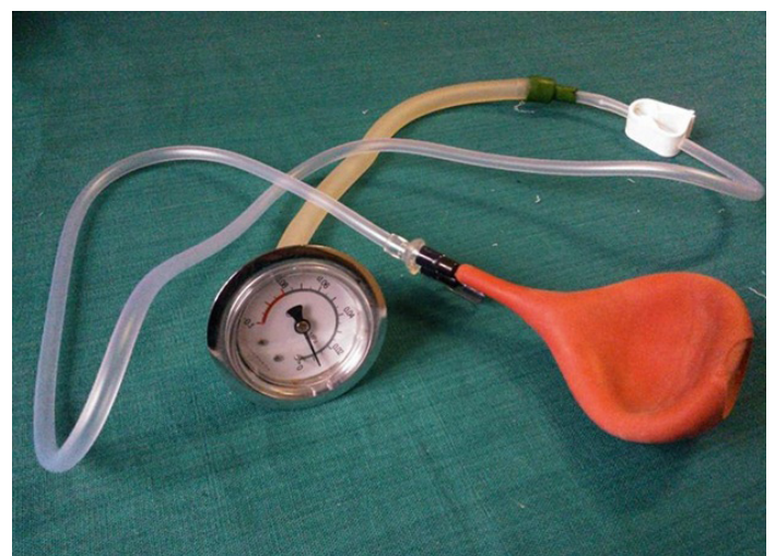
[Table/Fig-2]: Measurement of maximum negative pressure of mucus sucker showing around 70 mmHg
