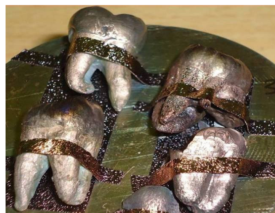
[Table/Fig-1]: Laboratory furnace (Model- BEGO@MIDITHERM) used in the present study. [Table/Fig-2]: Scanning electron microscope (Model-HITACHI S-3400N) used in the present study. [Table/Fig-3]: Incinerated teeth coated with gold of 600 Å thickness by low vacuum sputter technique for scanning electron microscopy.
