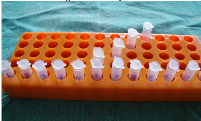
(Table/Fig 3) RBCs settle down at the bottom giving plasma supernatant
