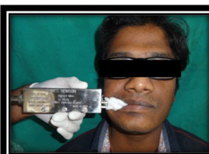
[Table/Fig-1]: Bite force sensor device containing a metallic sensor and a display monitor. [Table/Fig-2]: Recording the bite force tolerance value clinically.
